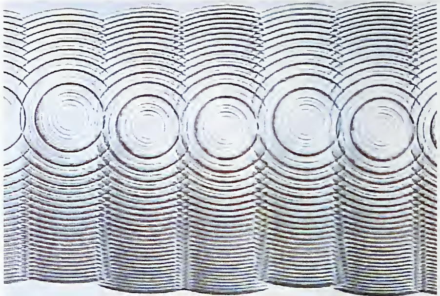
Photomicrograph of an array of multi-level diffractive lenses, fabricated with a 193 nanometer excimer laser.
